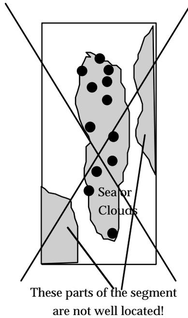
**Figure 6:** Example of a case where the attitude biases estimation is impossible: the visible parts of the image without ground control points (represented by black points) are not well located.
